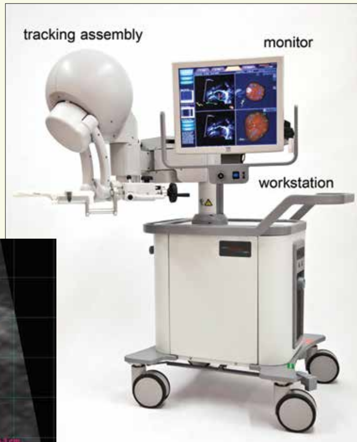
Figure 2. Artemis™ 3D ultrasound biopsy tracking system (Eigen, Grass Valley, CA). Reprinted from: Natarajan S, Marks LS, Margolis DJ, et al. Clinical application of a 3D ultrasound-guided prostate biopsy system. Urol Oncol 2011;29(3): 334-342. © 2011, used with permission from Elsevier.
