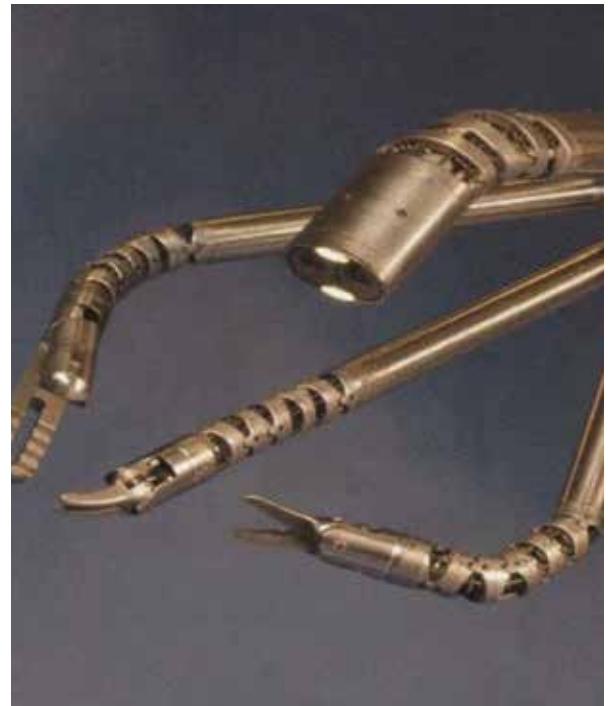
Figure 1. Novel robotic single-port arm. Common sheath houses two cameras for stereoscopic vision, light source, and three instruments that articulate at different levels for extended range of motion.
