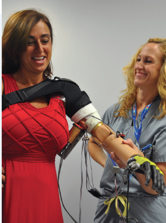
Figure 1. A neural-machine interface on this advanced prosthetic arm enables hand closure to be controlled by thought. The robotic hand also is equipped to provide sensory feedback to the user. (Photo by Paul Marasco, PhD.)
