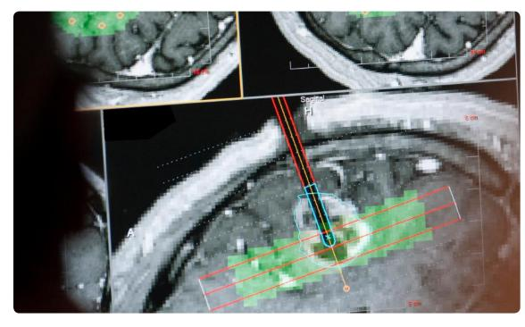
LEFT: MRI-guided stereotactic laser ablation using the NeuroBlate system.
