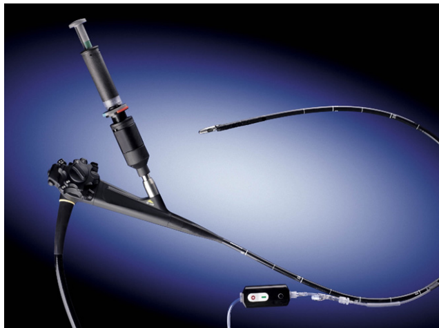
Fig. 1. Restore Suturing System uses a suction capsule placed on the end of a standard endoscope. Suction is applied to capsule using tubing attached to outside of endoscope. Suturing system and suture fastening system are operated through working channel of the endoscope. Multiple gastric plications can be completed with single esophageal intubation and no overtube.
