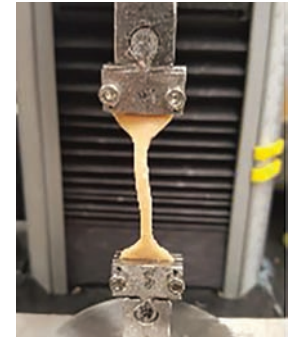
Uniaxial testing of extracted specimens to compare the in vivo and ex vivo mechanical properties of ascending aortic tissue in acute dissection vs nondissected tissue
